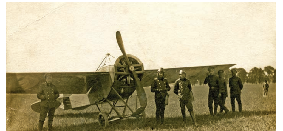
The Nieuport IV two-seater reconnaissance aircraft was one of the principal machines used by the Imperial Russian Air Service. Nearly 300 were produced under license in Russia by the Russo-Baltic Wagon Works in St. Petersburg and the Dux Factory in Moscow.
